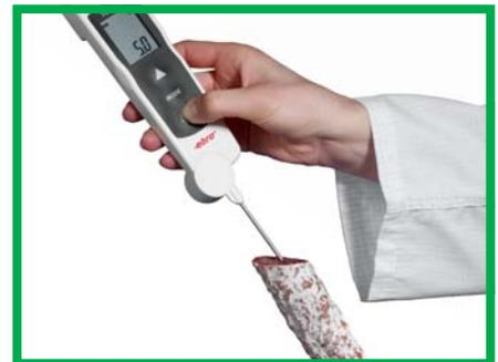
*Incorrect - the probe tip may not stick out of the measured good*
